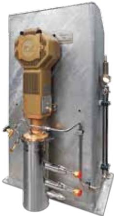
ACD's P2K reciprocating pump features a vertical design that offers less vibration, reduced noise, and a compact system footprint. Its cold end is submerged inside a vacuum-jacketed liquid sump, minimizing heat leak and increasing system efficiency.
