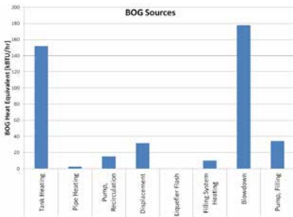
**Figure 1.** Relative magnitudes of the sources of heat leak in an example LNG production (N<sub>2</sub> cycle) and export terminal.
