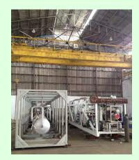
COLD BOX AND WARM END SHIP INSIDE 45 FOOT ISO CONTAINERS, COMPLETE WITH ALL PIPING, INSTRUMENT, ELECTRICAL AND INSTRUMENTATION
