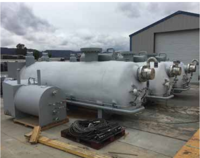
Figure 6 – Range of mobile natural gas fired vaporizers & trim heaters
