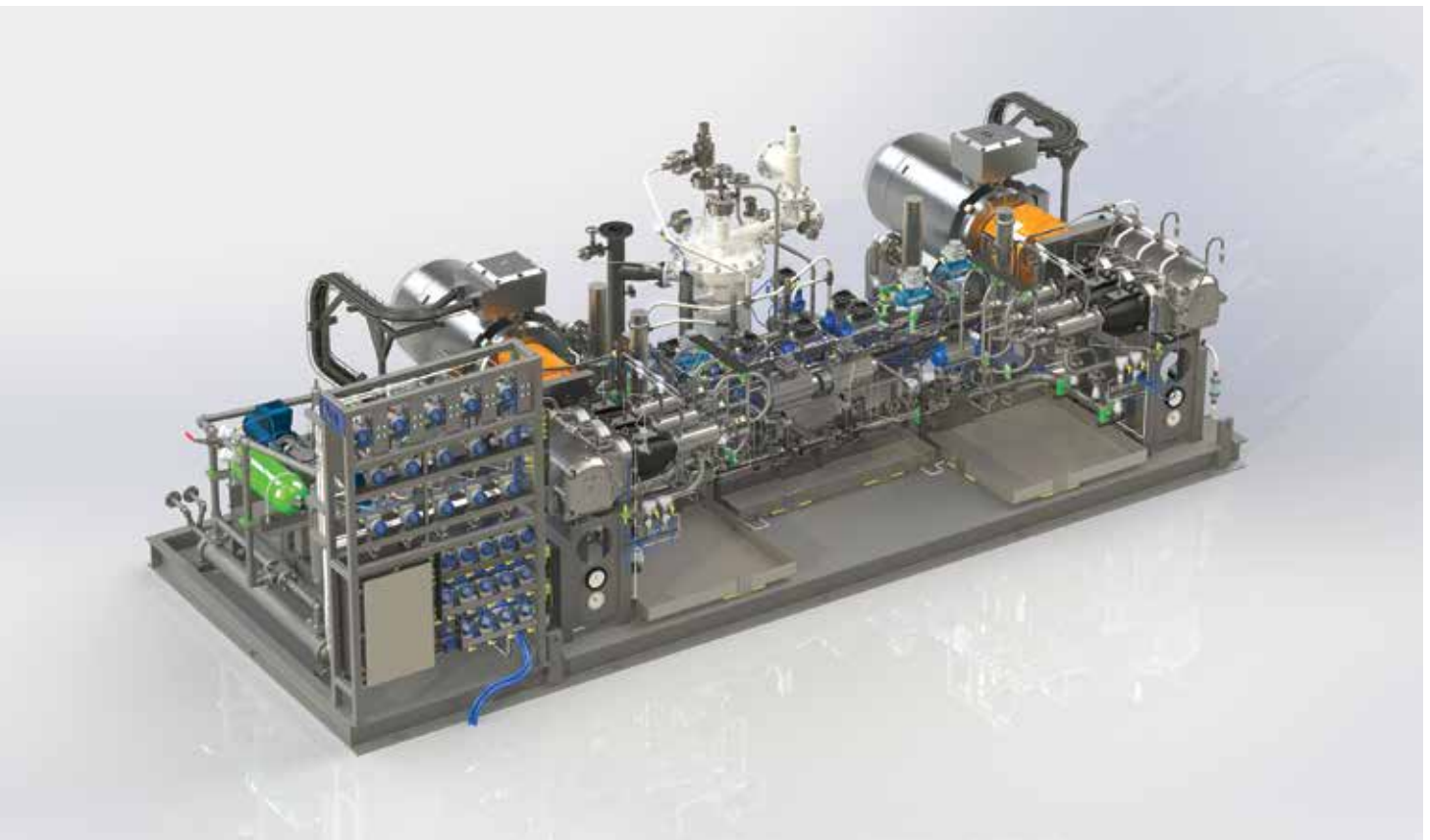
Figure 3: Shipboard high pressure fuel supply system
