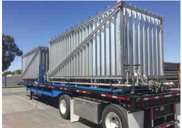
Figure 1- Trailer mounted natural draft ambient system
