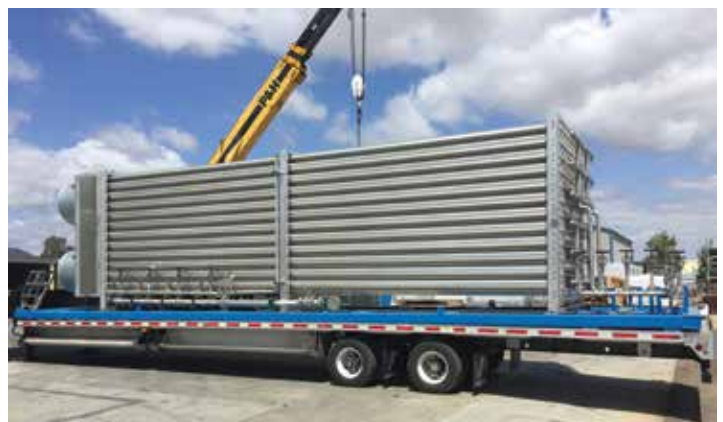
Figure 3 - Horizontal fan ambient vaporizer
