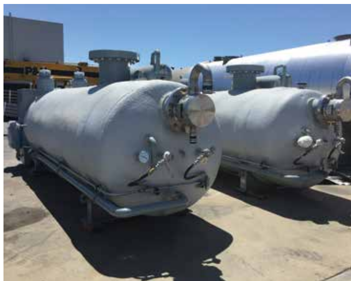
Figure 7 – Trailer mount natural gas fired water bath vaporizers
