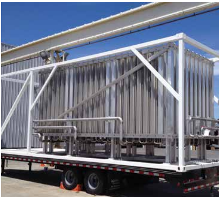
Figure 4 – Ambient with three circuits in one frame
