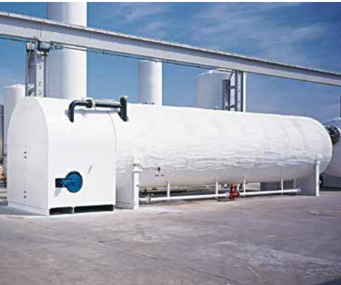
Figure 1: Natural Gas Fired Water Bath Vaporizers
