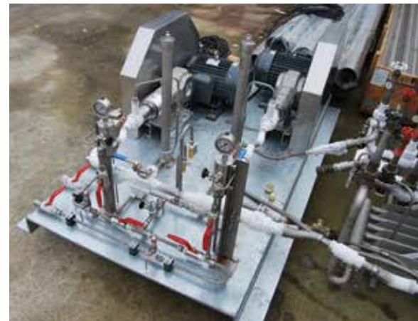
Figure 5: Dual RPSA-40 CO2 Cylinder Filling Skid
