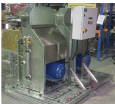
Figure 2: Dual P2K CO2 Well Injection Pump Skid
