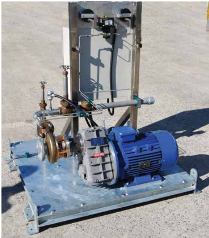
Figure 1: Simple TC-21 LOX Transfer Skid
