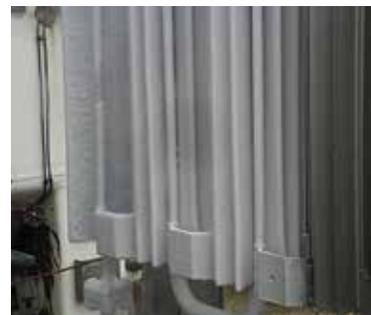
A frequent installation error occurs when installing hybrid ambient vaporizers. Hybrid ambient vaporizers have a variety of fin counts, some of the most common having a combination of 4-finned and 12-finned extrusions. Hybrids are typically used in long freeze
