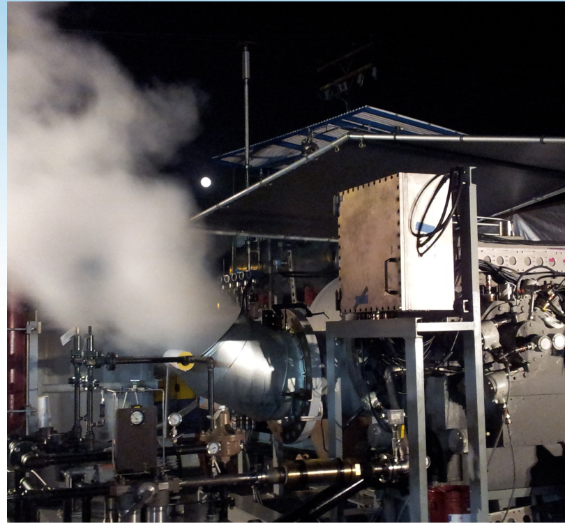
Figure 2: The turbine in operation during the 4 hour customer witnessed endurance test at night. The plume of gas with vapor can be seen exiting the turbine while the turbine operated at 13 650 rpm.
