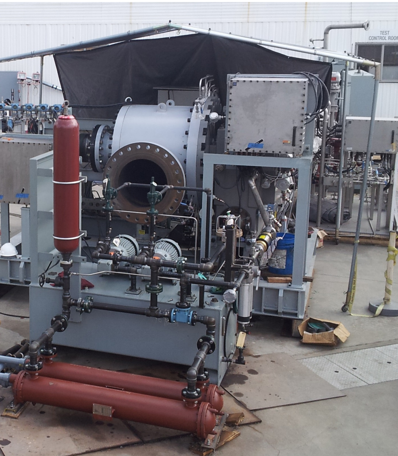
Figure 1: Test arrangement of a 4MW turbine only at the Santa Ana facility of Energent.
