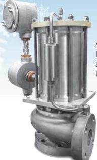
A II cryogenic pumps face two operational challenges. First is running two phase flow, that is supplying the pump with liquid close to its boiling point, and second is insufficient initial pump cool-down. Either case will lead to cavitation, resulting in pump damage and reduced life.
