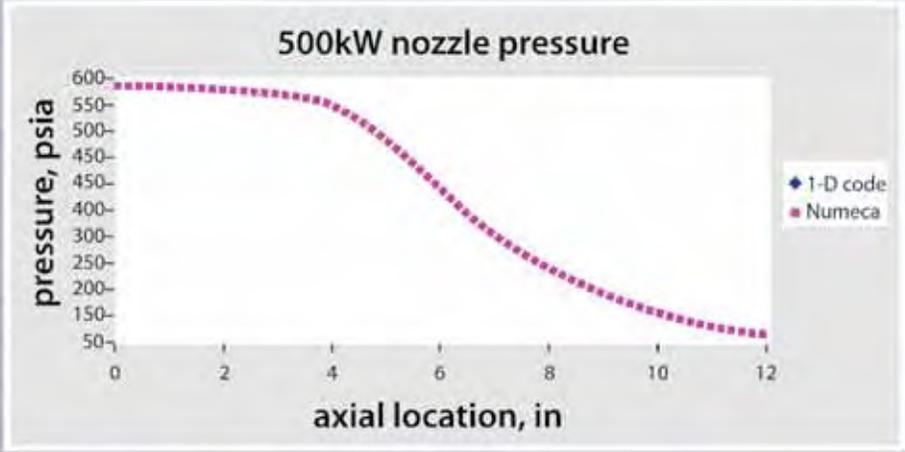
Figure 4. Pressure profile of a 500kW nozzle.
