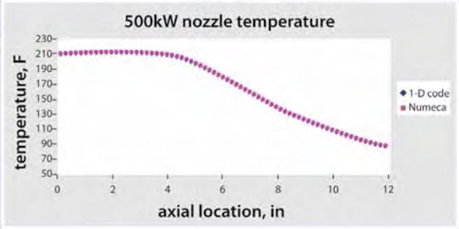
Figure 5. Temperature profile of a 500kW nozzle
