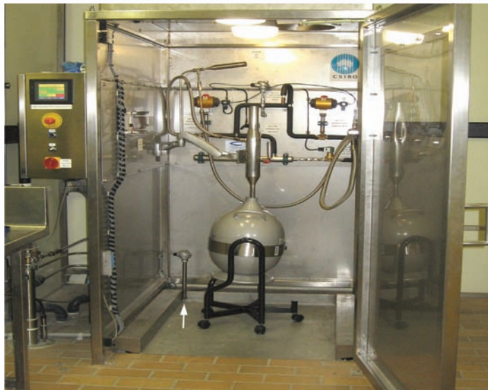
Figure 5: Overall view of \text{LN}_2 Dewar Filling Station. The Dewar is placed on a metal tray, where the weight of the Dewar is monitored. The metal tray is also equipped with a temperature sensor (white arrow), which will cease the flow of \text{LN}_2 in the event of a spill.
