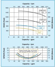
limited from the on-board power (pony engine or PTO) of the trailers. With designed maximum power capacity of 134 hp (100 Kw), the TOP 260 can reach differential pressures up to 1,475 ft (450m) and flows up to 290 gpm (1,100 lpm). For laser-fill applications where higher pressures are needed, the TOP 180-2s is available with maximum flows and pressures up to 225 gpm (850 lpm) and 2,200 ft (670 m) differential head, respectively.
