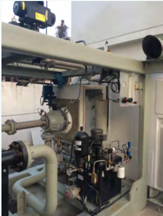
ACD TURBINE WITH LUBE OIL AND SEAL GAS
