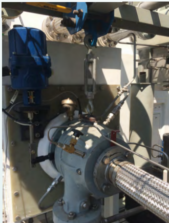
ACD TURBINE WITH LUBE OIL AND SEAL GAS
