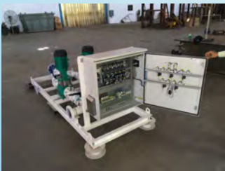
GLYCOL TO AIR DRY COOLING TOWER WITH PUMPS AND CONTROL, EXPANSION TANK
